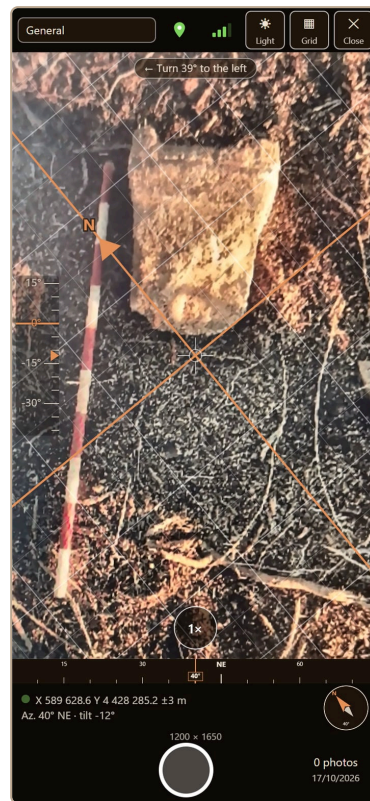
Figure 1. The BOIRA Survey viewfinder: active series, GPS status, crosshair, tilt, bearing strip with the north line, compass rose, and real-time coordinates and accuracy.
